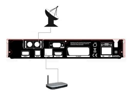
Figure 6. Connecting to Dish LNB
