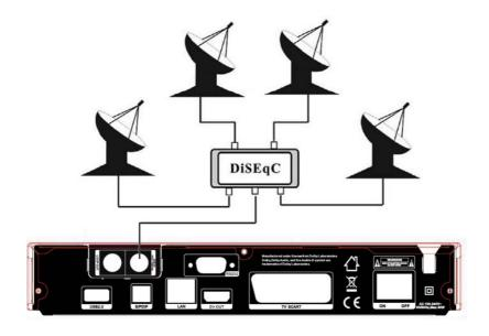
Figure7. Connecting to Dish LNB
