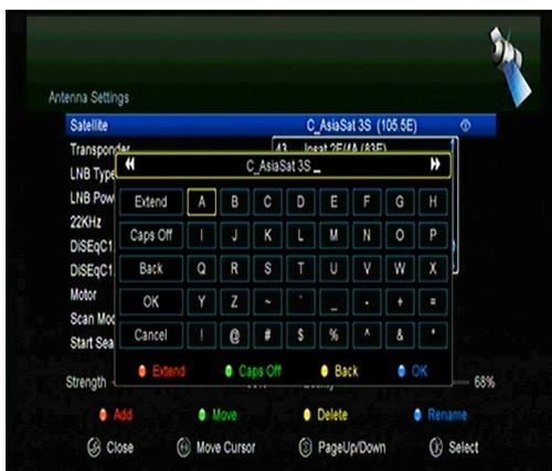
Transponder frequency, choose polarization (Ver, Hor), input new symbol rate, and **BLUE** choose FEC (1/2, 2/3, 3/4, 6/5, 7/8, Auto). **OK** to confirm the settings, and this new Transponder will be added to the TP list in ascend order sorted by frequency.
