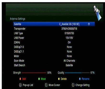
6. **DiSEqC 1.0:** Press the ◀/▶ button to select the required DiSEqC1.0 input.
