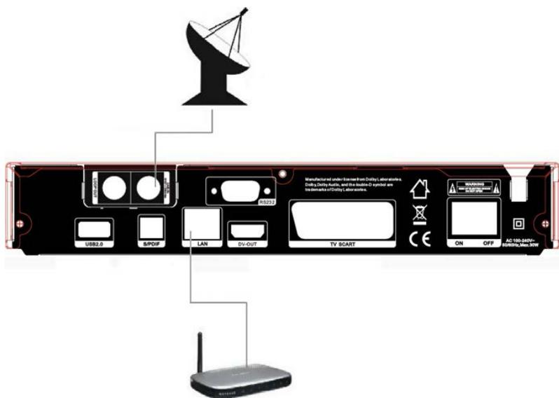
Figure6. Connecting to Dish LNB
