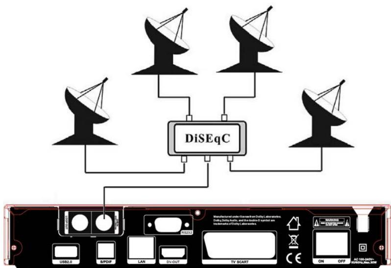
Figure7. Connecting to Dish LNB
